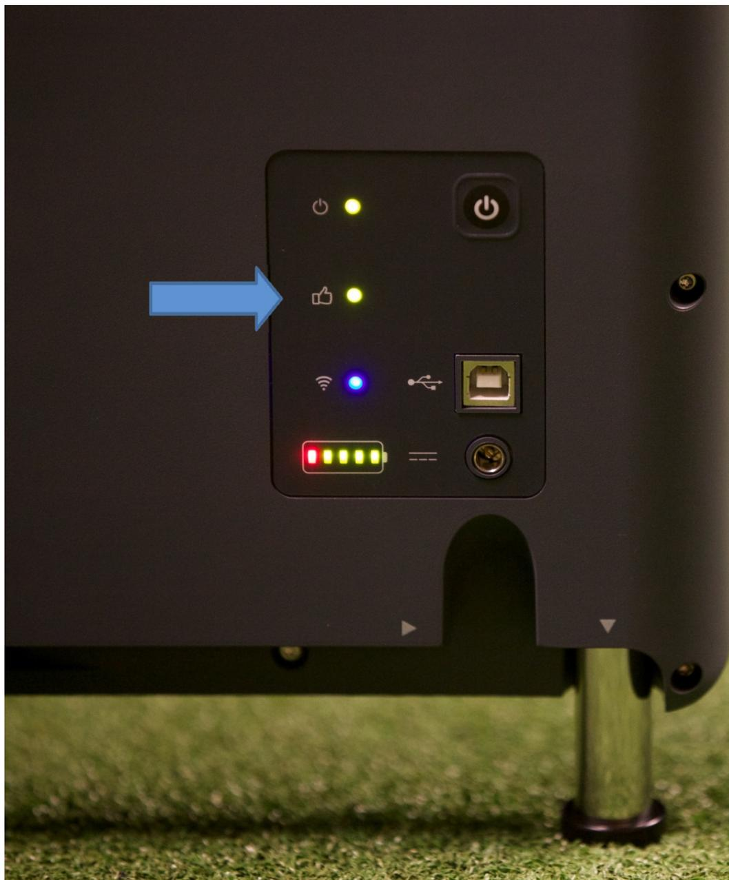
**Thumbs up means the system is armed and ready to collect data. If this LED is not on while in the Live tab of TPS, try clicking the Home tab and then going back to the Live tab.**
