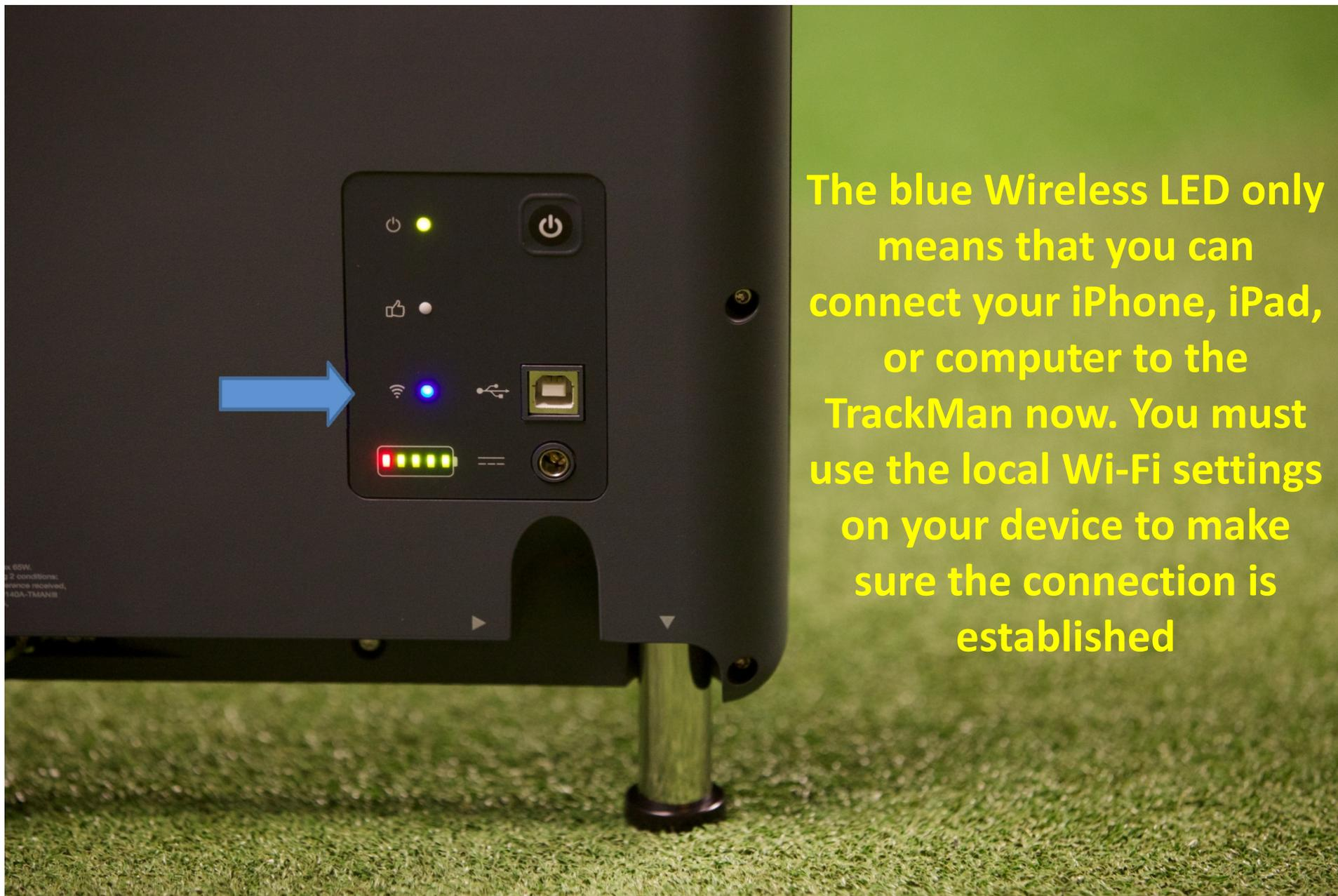
The blue Wireless LED only means that you can connect your iPhone, iPad, or computer to the TrackMan now. You must use the local Wi-Fi settings on your device to make sure the connection is established
