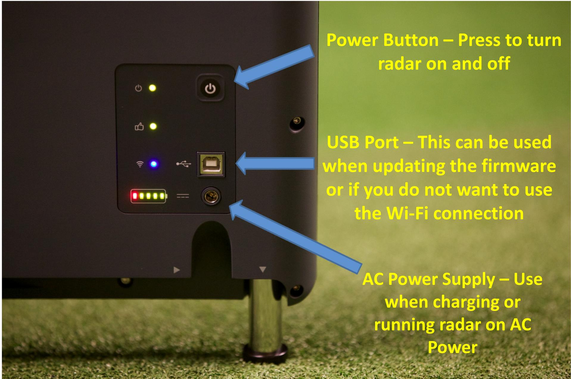
**Power Button – Press to turn radar on and off**
