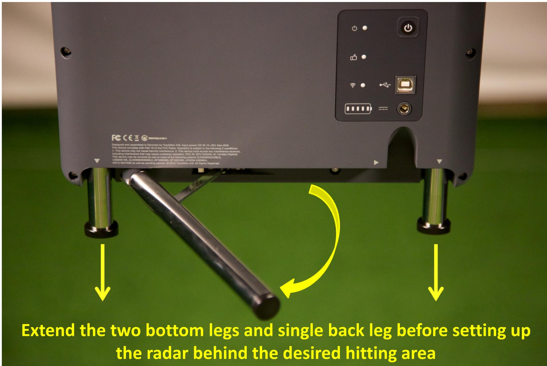
**1. There are two bottom legs that must be extended prior to setting up and turning on the radar. Pull the legs out until they click into place**
