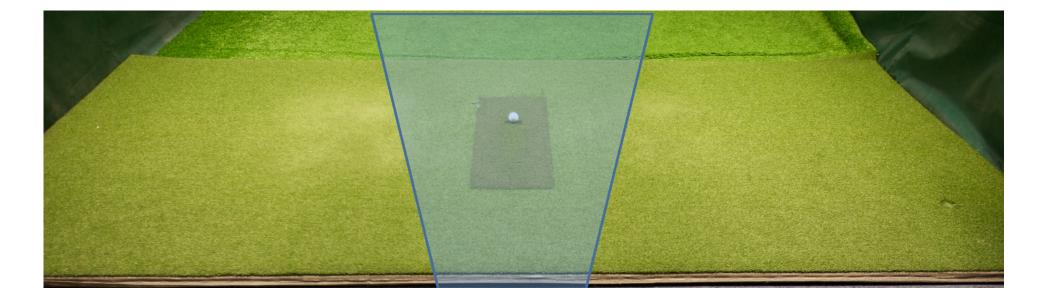
The actual view of the radar is 26 degrees (13 degrees on each side of center). This means that the further you are from the radar the more area you have right and left of the center line to capture data
