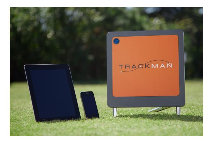
Extend the two bottom legs and single back leg before setting up the radar behind the desired hitting area
