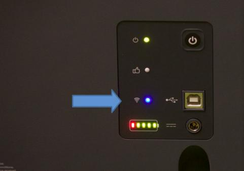
The blue Wireless LED only means that you can connect your iPhone, iPad, or computer to the TrackMan now. You must use the local Wi-Fi settings on your device to make sure the connection is established
