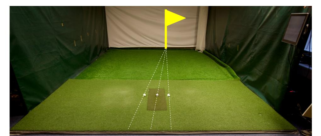
Data is measured relative to a target line that connects where the ball took off and the target chosen by the internal TrackMan camera
