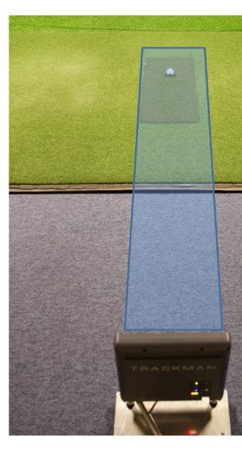
To increase club delivery pickup rate in certain situations, the radar can be moved slightly off of the target line and turned in to face the hitting area. This can allow the radar to see post impact club data better (example for right handed golfer)
