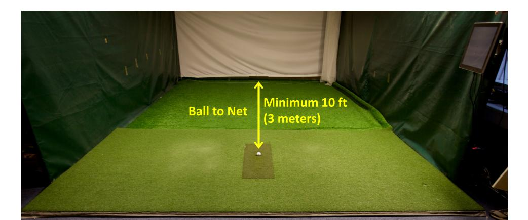
In order to measure Spin Rate in Indoor mode, it is recommended that you have a minimum of 10 feet or 3 meters of ball flight
